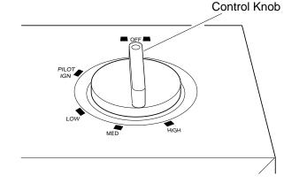
Figure 20 - Control Knob In The OFF Position
